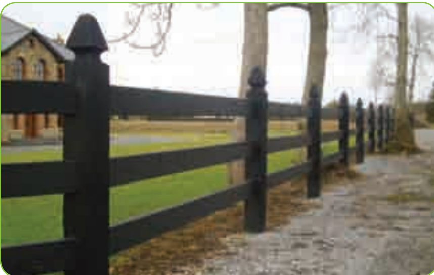
150mm x 150mm posts, 150mm x 44 rails
